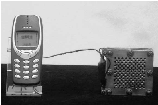
Fig. 11. Mobile phone powered by air-breathing DMFC cell pack.
